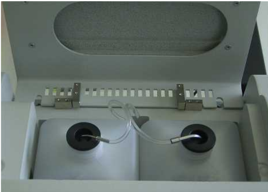
fig. 6.5 view of supply and waste container
